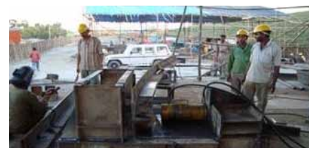
Fig-13: Bending of the ISA 200X200X20
